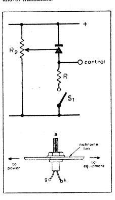
The heating element can be isolated from the thyristor case, or it can be a short resistive link, in the positive line or bolted to a heat sink, and connected to the thyristor anode as shown. In d.c. circuits a  $1/25\Omega$  will monitor a 25A circuit with ease. Thyristor packaging and mounting govern the thermal inertia of the system.
